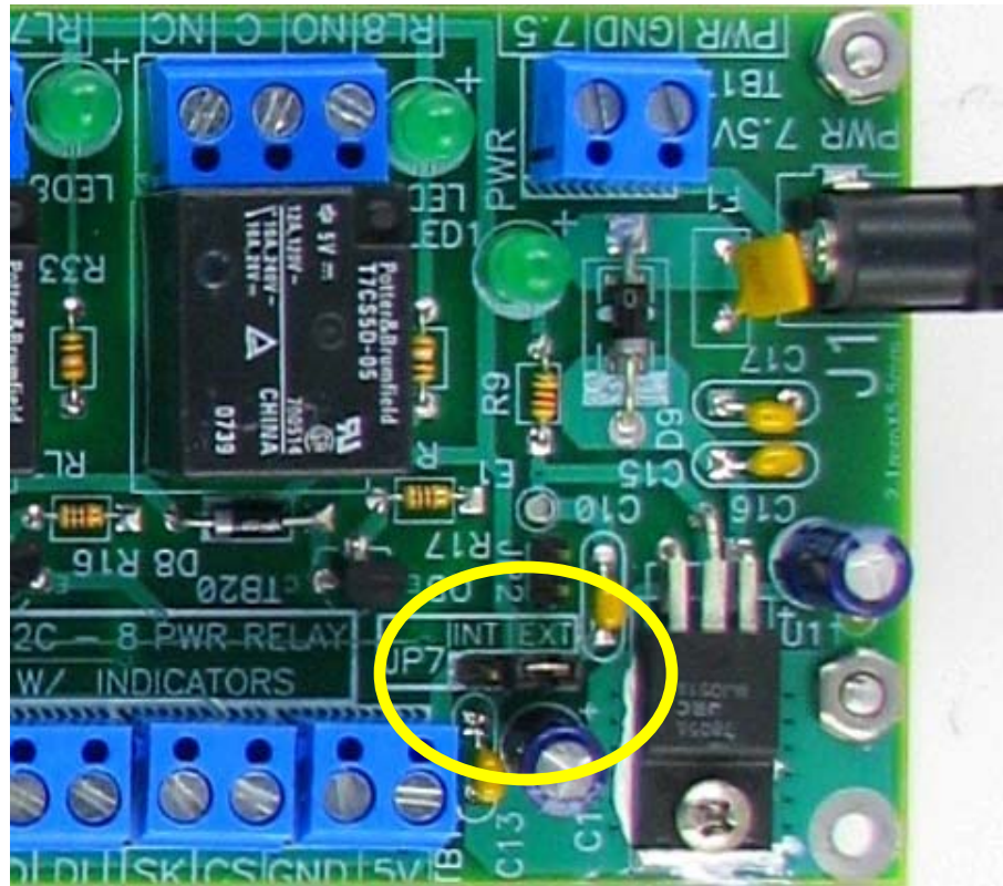
Figure 4: Power Jumper JP7. “INT” means power from the I2C port, “EXT” means power from the DIN connector J1 or terminal block TB17.
