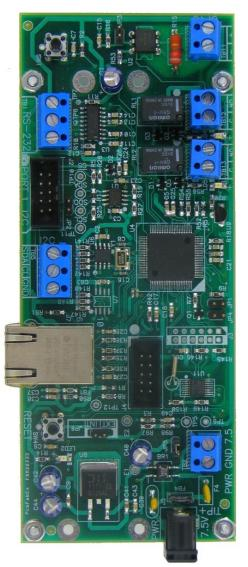
USB/I2C/RS232 Tester (KA-I2C-RS232-TEST) Web-Accessible I/O Card (KA-WEB-I2C-TH)
