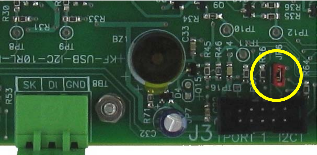
Figure 5: I2C Jumper JP6.
