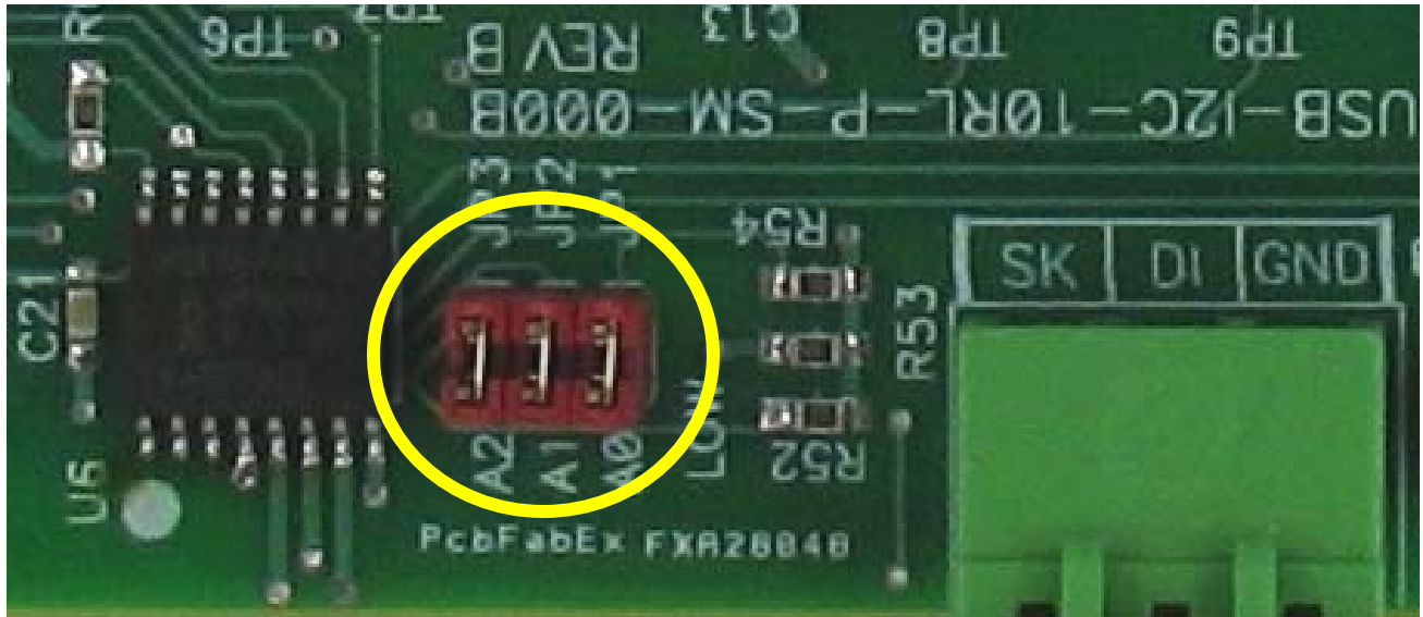
Figure 6: I2C Address Jumpers JP1-JP3.
