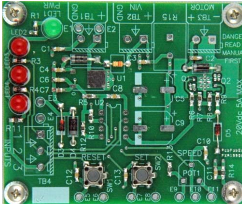
Figure 13: Board with push-button switches installed.
