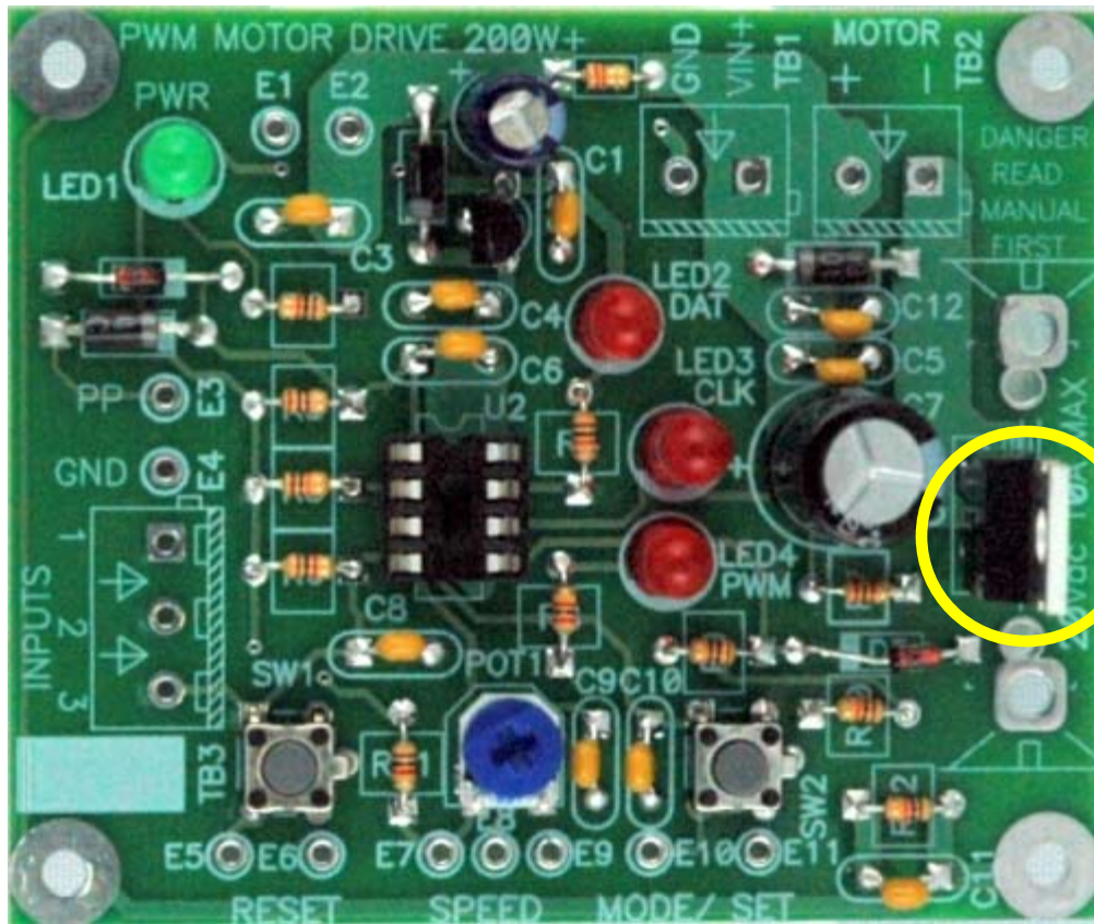
Figure 17: Board with MOSFET installed.
