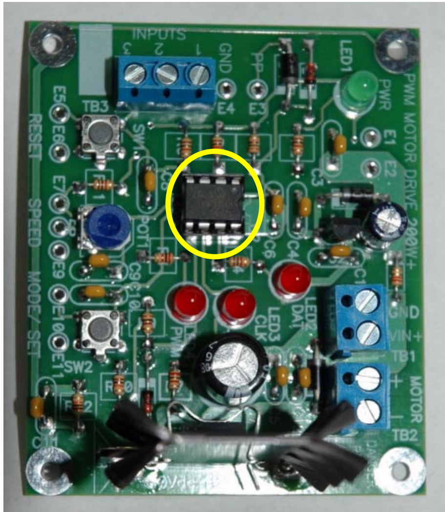
Figure 20: Board with socket and processor installed.
