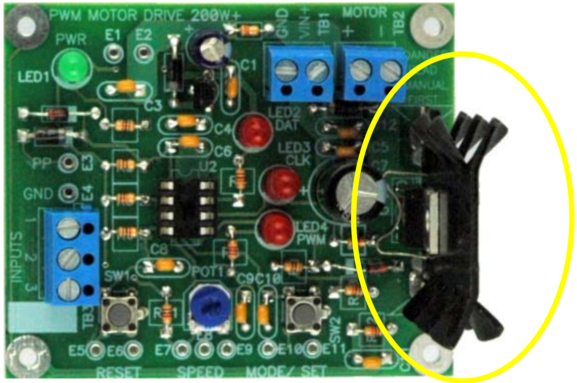
Figure 18: Board with heat sink installed. Optional heat sink in some kits
